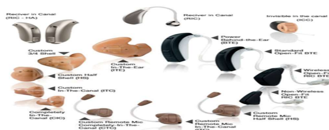
Figure-8: Different types of hearing aids
