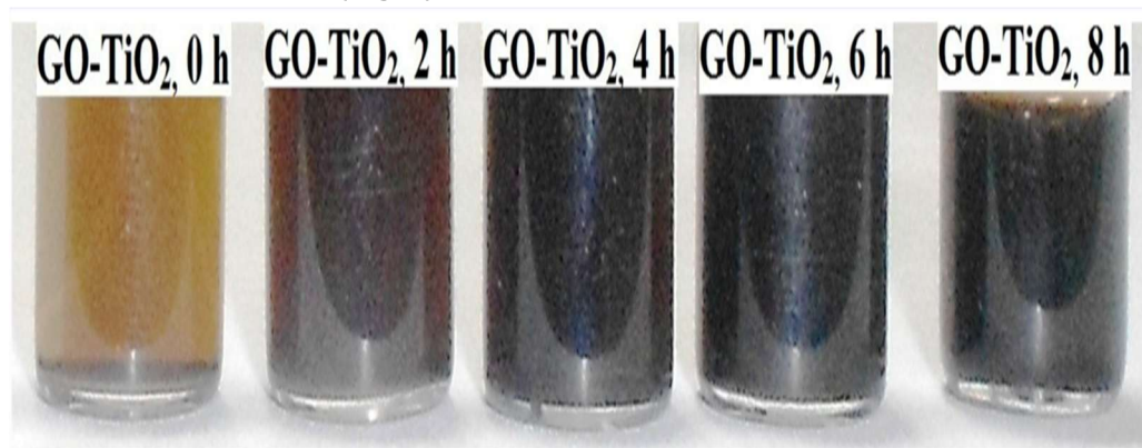
Fig. 3. Digital image of UV light (0, 2, 4, 6, 8 h) irradiated GO-TiO 2 nanocomposite solution
